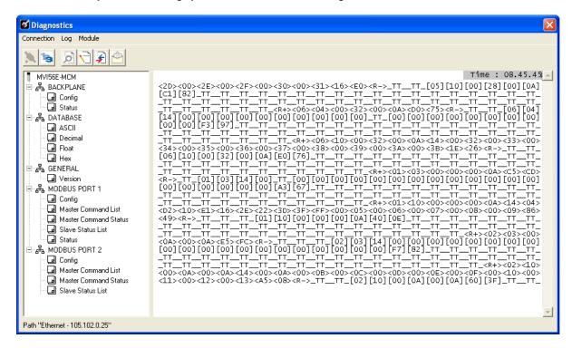
The <R+> means that the module is transitioning the communications line to a transmit state.
