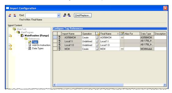
**10** Associate the I/O connection variables to the correct module. The default values are Local:1:I and Local:1:O so you may have to edit the **FINAL NAME** field to change the values. You can also click the drop-down arrow to select the correct name.
