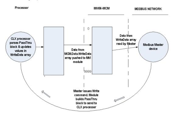
**Note:** For RSLogix version 15 and lower, the ladder logic necessary for the successful execution of this block is contained in the subroutine PassThru.
