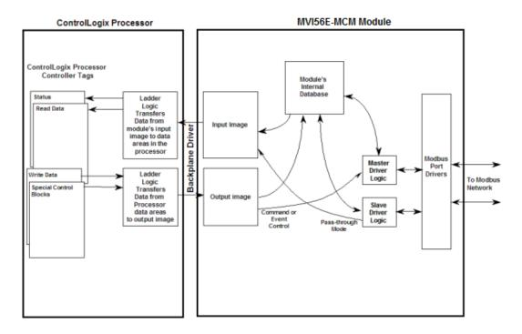
As shown in the illustration above, all data transferred between the module and the processor over the backplane is through the input and output images. Ladder logic must be written in the ControlLogix processor to interface the input and output image data with data defined in the Controller Tags. All data used by the module is stored in its internal database. This database is defined as a virtual Modbus data table with addresses from 0 to 15999.
