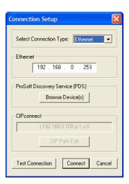
You can also use CIPconnect® to connect to the module through a 1756-ENBT card by choosing 1756-ENBT in the **Select Connection Type** list Refer to Using CIPconnect to Connect to the Module for information on how to construct a CIP path.
