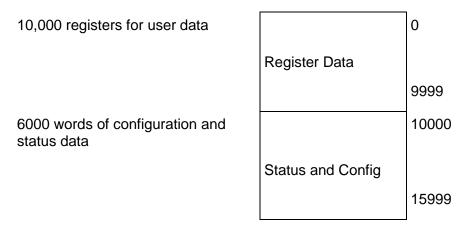
Data contained in this database is paged through the input and output images by coordination of the ControlLogix ladder logic and the MVI56E-MCM module's program. Up to 248 words of data can be transferred from the module to the processor at a time. Up to 247 words of data can be transferred from the processor to the module. Each image has a defined structure depending on the data content and the function of the data transfer as defined below.
