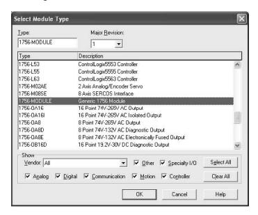
3 In the MODULE PROPERTIES dialog box, enter the Name, Description and Slot options for your application, using the examples in the following illustration. You must select the Comm Format as DATA - INT in the dialog box. Failure to set the correct parameters will result in backplane communication problems between the module and the processor.
