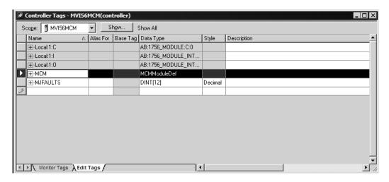
5 Drag the **MCM** tag structure to the blank line at the bottom of the list in the **EDIT TAGS** tab in your existing program.
