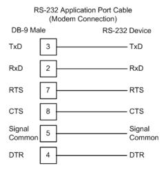
The "Use CTS Line" parameter for the port configuration should be set to 'Y' for most modem applications.
