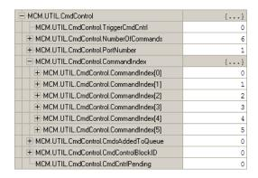
The following configuration will place 6 commands into the command queue. **MCM.CONFIG.Port1MasterCmd[0]** to **MCM.CONFIG.Port1MasterCmd[5]** will be enabled with this configuration. Error codes for each command are placed in the Error Status table.
