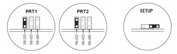
The Setup Jumper acts as "write protection" for the module's firmware. In "write protected" mode, the Setup pins are not connected, and the module's firmware cannot be overwritten. The module is shipped with the Setup jumper OFF. If you need to update the firmware, apply the Setup jumper to both pins.
