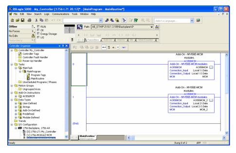
The setup procedure is now complete. Save the project and download the application to your ControlLogix processor.
