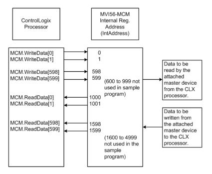
The sample configuration values configure the module database for **WRITEDATA[0 TO 599]** to be stored in the module memory at register 0 to 599, and **READDATA[0 TO 599]** to be stored in the module memory at registers 1000 to 1599 as shown above.
